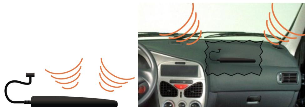
The tracker should be fixed on the top side (with LEDs) facing up, to "looking at the sky." Always add silicone glue or tape double-sided at the base of the equipment.
